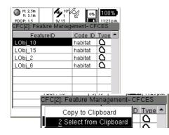
Areas internal to the main feature, or parent area, can be excluded from the calculation. The selection process is identical to selecting a main feature, but it is possible to select multiple features to be excluded. The 09 command will not only provide the number of features excluded, but will provide detail about each feature.
